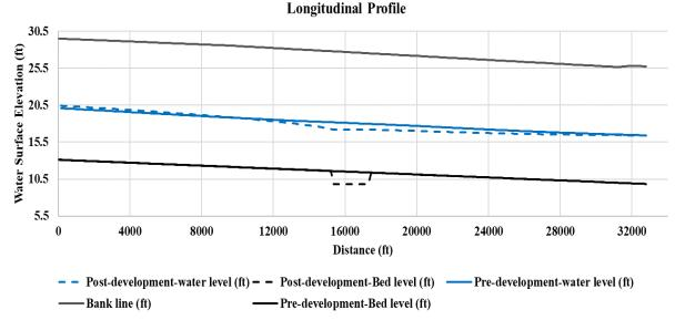
post- conditions, pre- and post- bed elevation (showing the detention facility), and left and right banks.
