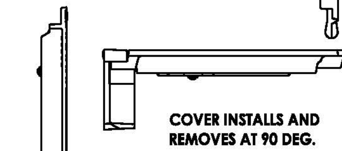
COVER AT 90 DEG. SAFETY STOP POSITION
